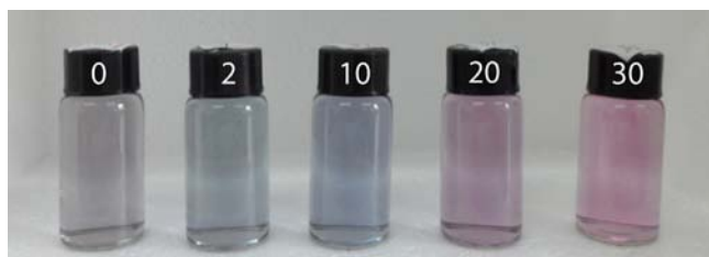
Fig. 3. Color responses when 0.75 mM AuNRs react with \text{Fe}^{3+} (from left to right: 0, 2, 10, 20, 30 \mu\text{M} ) system containing 2.50 mM \text{H}_2\text{O}_2 and 30.0 mM HCl at 70 °C for 25 min under pH 1.55.
